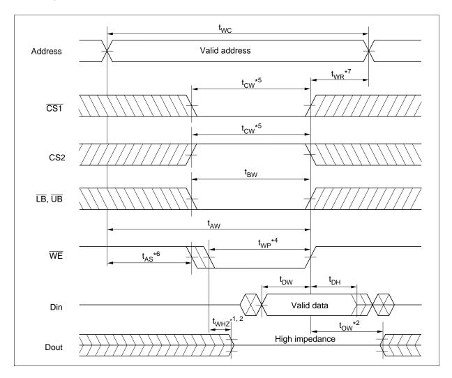
Write Cycle (2) ( $\overline{\text{CS}}$  Clock,  $\overline{\text{OE}} = V_{\text{IH}}$ )
